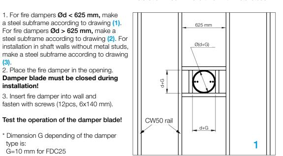
FDC-MF2 Fire damper (Ød > 625 mm) installation in 90 mm shaft wall with metal studs
