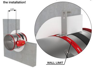
The damper driving mechanism can be placed on either side of the wall, however it needs to be placed so that it ensures an easy access during inspection.
