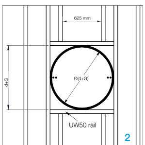
FDC-MF2 Fire damper installation in 90 mm shaft wall without metal studs
